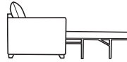
2/3 Seater sofas Two fold slatted and webbed metal action. Depth open 2280mm
